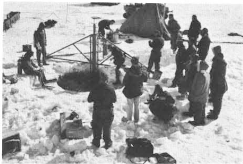
THE HOLE THING—Ice melter device is readied for test. Right: A diver goes below to photograph bottom of ice.
