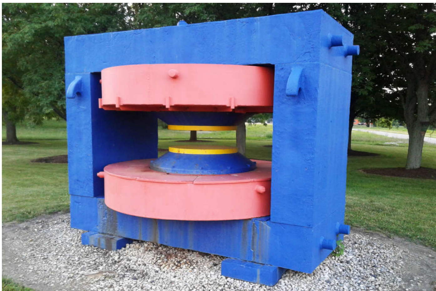
The magnet yoke from a cyclotron, built in 1935 by Professor William D. Harkins and colleagues at the University of Chicago [187]
