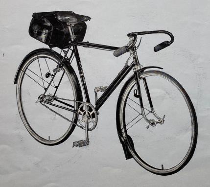
Frame. Sizes 20", 21", 22" and 23". built entirely from "SUN" Lugs of upright design, with 71° seat tube. 3/16" balls in bottom Head lug. 531 tubing. All brazed on mudguard eyes, pump pegs, etc. Solid front
